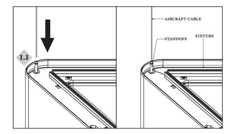
1.1 FROM THE TOP OF THE FIXTURE, INSERT EACH AIRCRAFT CABLE INTO THE STANDOFF UNTIL THE DESIRED HEIGHT IS ACHIEVED.
