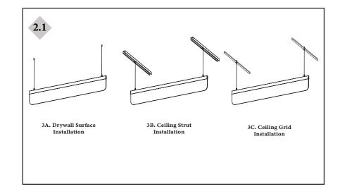
2.1 TO PROPERLY INSTALL THE FIXTURE REFERENCE 3A, 3B, OR 3C TO COMPLETE THE INSTALLATION DEPENDING ON THE SURFACE TYPE. **STEP 3A**
